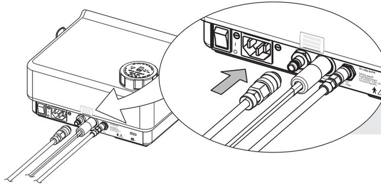
Use only dry, pure, and filtered compressed air.
